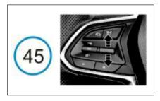
The expected cruise speed is displayed on the combined instrument.
