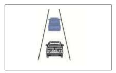
The vehicle in front that is followed by this vehicle will be displayed in the form of blue graphic in the instrument.
