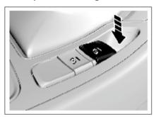
If you have to release parking brake, firstly confirm that the ignition switch is at the ON position, depress the brake pedal, and then press the EPB switch. The EPB working indicator goes out, and the instrument cluster displays "parking brake released", reminding you of parking brake released.
