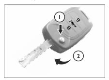
As shown in the figure, press the release button, and the mechanical key will pop up automatically.
