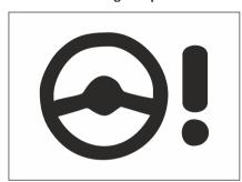
This warning lamp will illuminate immediately the ignition switch is turned on. It indicates that the system is conducting self-inspection and the warning lamp bulb can work normally. The warning lamp goes out several seconds later.
