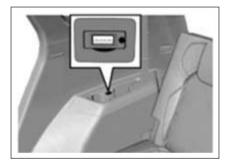
There is USB power jacks (5V/2A) available for the second and third row sea t and can be used for charging mobile phones. The power is not available when the vehicle ignition switch is off.Warning Lamps, Gauges and Indicators
