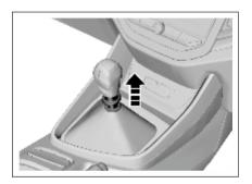
As shown in the figure above, when shifting the transmission with six drive gears to the reverse (R) gear, pull up the reverse gear lock ring firstly and then turn the gear lever from the neutral (N) gear to the reverse (R) gear. Take care not to pull the reverse gear lock ring when shifting to the drive gear, so as to avoid from shifting to the reverse gear accidentally.
