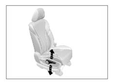
Turn the handle on the outer side of the seat upward and downward until the seat is adjusted to the desired height. While adjusting the seat height, the seat must be loaded. Therefore, please sit on the seat before adjustment; otherwise the adjustment device may be damaged.
