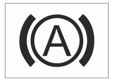
The automatic vehicle hold (AVH) working indicator illuminates after the ignition switch is turned on and it goes out several seconds later. This indicates that the indicator can work normally. For certain vehicle models, the indicator does not illuminate when the ignition switch is turned on.
