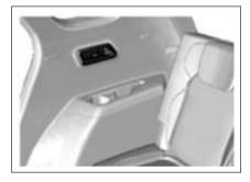
There is two rear air outlet for the 7 seater variant. You can decide the flow direction from the adjustable air outlet.
