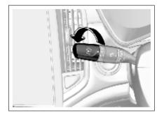
When the headlamp is in low beam state or the front fog lamp is turned on, turn the rear wiper control knob to "s" position and then release it to turn on the rear fog lamp. Turn the knob again to turn off the rear fog lamp.
