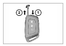
As shown in the figure above, turn the release switch ① on the key first, and then pull out the mechanical key ②.
