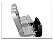
As shown in the figure, after the cushion is unlocked, pull out the cushion forward and lift up the rear part of the cushion to overturn it. The two cushions can all be overturned.
