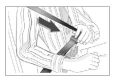
I. Pull out the seat belt from the recoiler, and fasten it across the body without twisting.
