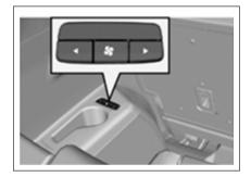
The switch located at the left rear cup holder for the 7 seater variant. Press the air conditioner switch tu turn on/off the A/C. You can press the arrow button to raise or lower the air volume for ther rear air outlet.
