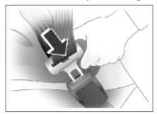
Put the latch plate in the buckle for fixing. Pull the shoulder belt forcibly to adjust the tightness degree of hip belt.
