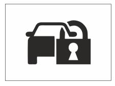
This indicator illuminates when the door is opened. It goes out after the engine is started. This indicates that the indicator can work normally. Refer to information on engine immobilizer system given in "Driving and Controls".
