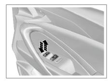
To raise the window, pull upward the switch. To lower the window, press down the switch. When the window reaches the desired position, release the switch.
