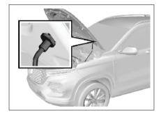
Separate the engine hood prop rod from the fixing clamp. Plug the free end of the prop rod in the slot.
