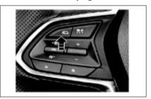
The driver can shortly press down the ( ) ON/OFF button on the steering wheel so as to activate the Lane Keeping Assist. At this time, the indicator light ( ) on the combined instrument is lit on, and the lane line turns gray in the indicator light. The system is in standby state.
