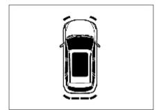
As is shown in the figure, when the transmission is engaged on the Forward Gear (D Mode) or the Neutral Gear, a prompt window will pop up in the audio system display screen as front end of the vehicle is within about 0.6 m from the obstacle or rear end of the vehicle is within about 1.5 m from the obstacle.
