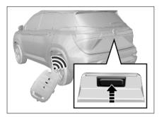
When the doors are locked and the ignition switch is at LOCK position, bring a legal key and get close to the liftgate (within 1.2 m); press the liftgate release switch, and the
