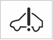
This indicator will illuminate when the 48V hybrid system not working.
