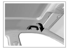
Above the front passenger's side door and rear doors, an auxiliary handrail is installed. The handrail of some models is equipped with a clothes hook.
