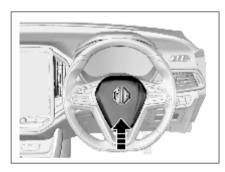
Press the switch on the steering wheel to blowthe horn.
