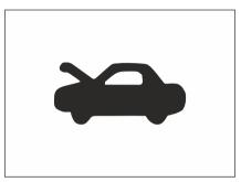
This indicator will illuminate when the engine hood is opened or it is not properly closed.
