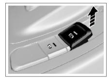
If you have to apply parking brake, depress the brake pedal to stop the vehicle and then draw back the electronic parking brake switch. In this case, the EPB working indicator illuminates, and you release the EPB switch after the instrument cluster displays "Parking brake applied".
