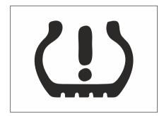
The warning lamp illuminates after the ignition switch is turned on and it goes out several seconds later. This indicates that the warning lamp can work normally.
