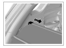
As shown in the figure, press the caps on both ends of the luggage cover recoiler toward the middle to remove the luggage cover from the vehicle.
