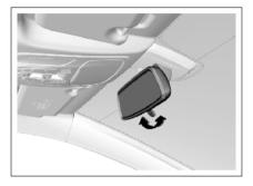
Adjust the rearview mirror to an appropriate angle manually. The rearview mirror of some models has anti-dazzling function which can reduce the dazzling effect from vehicles behind at night. Turn the switch at the rearview mirror bottom forward to activate the antidazzling mode. Please remember to turn the switch back at day time.
