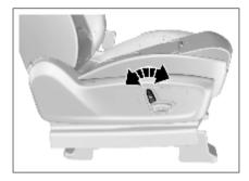
As shown in the figure, turn the adjustment switch forward and backward, and the backrest will be folded forward or unfolded backward. Release the switch when it is adjusted to a proper position.
