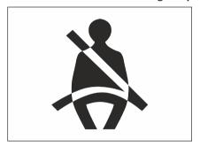
The seat belt warning lamp illuminates if the driver does not fasten the seat belt properly after the ignition switch is turned on. Following this, the following circumstances will appear unless the driver fastens the seat belt properly:
