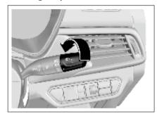
When the ignition switch is turned to ON position, and the headlamp functions as a position lamp or in a low beam state, turn the ring button in the middle of the combination switch to ON (connected) position to turn on the front fog lamp. Turn the ring switch to OFF (disconnected) position to turn off the front fog lamp.
