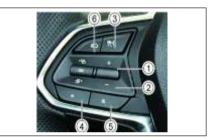
Press the ACC buton on steering once to activate the ACC (highlighted by no. 3) Other functions of the ACC switch are as follows
