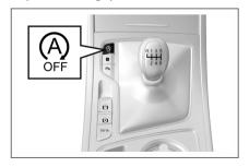
After starting the engine, press the start-stop disabling switch, as shown in the figure. The start-stop system OFF indicator on the instrument cluster turns on, and the start-stop function is disabled. Press the switch again to enable the start-stop function again.
