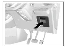
The indoor fuse box is on the lower right side of the instrument panel and it can be seen after pulling out the storage box.
