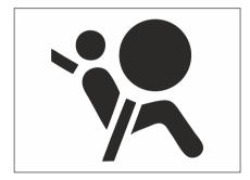
On the instrument panel, there is an air bag indicator which displays the air bag shape symbol. The system will check whether the air bag circuit system has a fault and give corresponding prompt through the indicator. Refer to the Chapter "Instruments and Controls" for detailed information.
