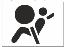
The airbag warning lamp illuminates when the ignition switch is turned on and it goes out several seconds later. This indicates that both the warning lamp bulb and the airbag system can work normally.
