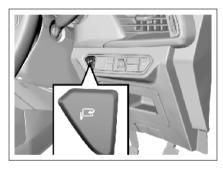
Press the electric folding button to fold the outside rearview mirror automatically.
