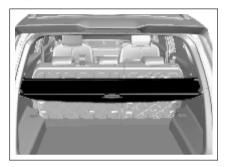
The cover is used to shield the objects in the luggage compartment.
