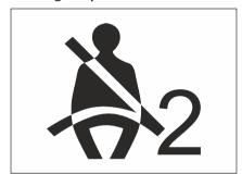
The seat belt warning lamp illuminates if the front passenger seat is occupied but the occupant does not fasten the seat belt properly after the ignition switch is turned on. Following this, the following circumstances will appear unless the front passenger fastens the seat belt properly:
