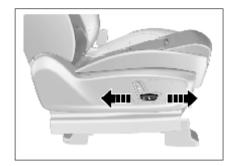
As shown in the figure, the electric adjustment switch is on the outer side of the seat. Push the switch forward or backward, and the seat will move forward or backward accordingly. Release the switch when it reaches a proper position.
