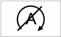
This indicator illuminates when vehicle start / stop function is not functioning.
