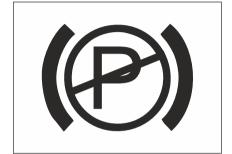
The electronic parking brake fault warning lamp illuminates after the ignition switch is turned on and it goes out several seconds later. This indicates that both the warning lamp and the electronic parking brake function module can work normally.
