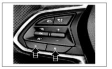
Press the left or right button of the toggle button so as to decrease or increase the following time interval.
