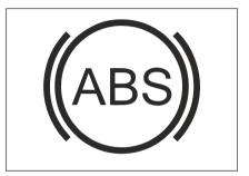
The ABS warning lamp will illuminate immediately the ignition switch is turned on. It indicates that the system is conducting self-inspection and the warning lamp bulb can work normally. The warning lamp goes out several seconds later.
