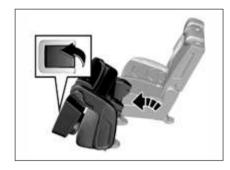
For the 7 seater variant, when you need to sit at the rear seat you can overturn the left side of middle row seat. As shown in the figure, you can pull the lever until the seat lock is detached. To recover, pull up the lever and push back the seat until it safely locked in position.
