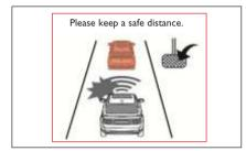
The Safe Distance Warning detects the vehicle in front via radar and provides the prompt message in the instrument in case of too-close distance between the vehicle and the vehicle in front.
