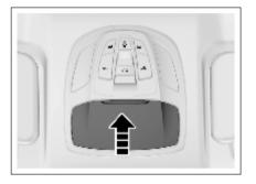
If equipped, the glasses box is located on the roof.
