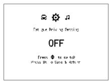
Enter the fatigue driving function setup interface and you can make fatigue driving function setup. Once the driving time reaches or exceeds the set value, a text warning message will appear on the LCD, accompanied by a sound alarm. The system reminds you to have a rest if necessary in this way. You can also disable the fatigue driving function by selecting the corresponding option on this interface. The fatigue driving function gets disabled by fault once the battery power is cut off.
