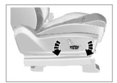
As shown in the figure, rotate the height adjustment switch on the outer side of the seat cushion, and then release the switch after the seat is adjusted to proper height.
