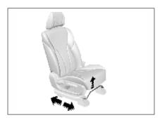
Pull upward the adjustment lever on the front lower part of the seat to adjust the seat forward or backward, and release the lever after the seat is adjusted to a proper position.
