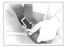
To unbuckle the seat belt, please press the red button on the buckle.
