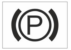
The electronic parking brake (EPB) working indicator illuminates as the electronic parking brake is pulled up. This indicates that the vehicle is in a parking state.
