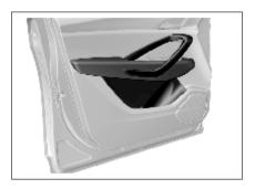
The door storage groove and armrest are located on inner side of the door panel.
