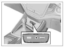
The entertainment system interface is located below the air conditioning panel. USB interface specification is 5V/2A, can be connected to play audio, charging. Power will not be available for charging when the vehicle ignition switch is off.
