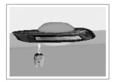
To lock a door outside of the vehicle with a key, plug the key and rotate it clockwise.
