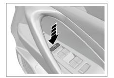
The power window lock button can lock the front passenger's side and rear power window switches. Press the button, and other power window switches are locked. The windows can only be operated with the driver's side window control panel.
