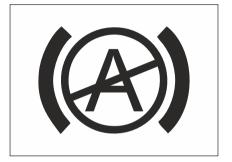
The automatic vehicle hold (AVH) fault warning lamp illuminates after the ignition switch is turned on and it goes out several seconds later. This indicates that both the warning lamp and the automatic vehicle hold function module can work normally. For certain vehicle models, the warning lamp does not illuminate when the ignition switch is turned on.
