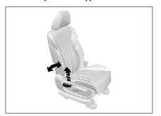
Pull up the handle near the seat cushion; adjust the backrest inclination angle to a proper position; then, release the handle. Please do not lean on the seat backrest while adjusting. After adjusting the seat backrest, try to shake the backrest to ensure that the backrest is locked.
