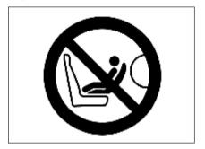
Do not use a backward-facing child restraint system on a seat (front seat) protected by a frontal air bag (in activated state). Otherwise, severe injuries or even death may be caused to the child when the air bag is deployed.
