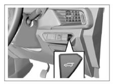
Press the switch. The liftgate automatically opens after two prompt tones. When the liftgate is to be closed, press the switch. The liftgate automatically closes after two prompt tones. The locking sound and two flashes of hazard warning lamp represent that the liftgate is closed and locked.
