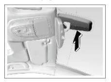
The sensor is installed on the front windshield Light and rain sensors are used to sense light and rain. The control module provides sensing signals for bad / good lighting & amount of water vapor / rainfall on the surface of the glass.
