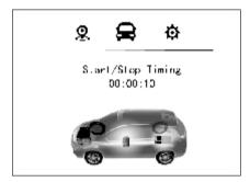
The start-stop timing displays the accumulated time of the auto engine stop after the ignition switch is switched on.
