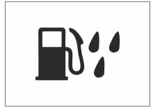
This indicator will illuminate when the water is mixed with the fuel.
