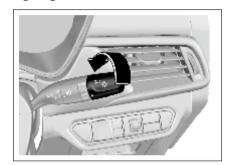
To switch ON or OFF the headlamp, tail lamp and parking lamp, please turn the end of the combination switch control lever.
